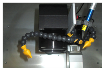
Sorgente laser con testa scanner Laser source with scanner head
