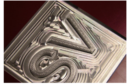
Stampo in magnesio Magnesium mold
